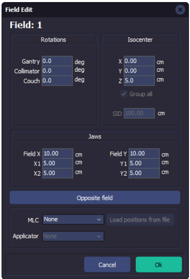
Figure 5.1: Field edit dialog. Changing the SSD to 95 cm. Notice that to set a SSD of 95 cm the isocenter must be located at 5 cm below the phantom surface.
